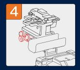
Fix the cleaver with the screw
