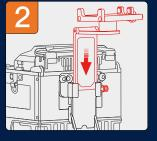
Insert into the base and tighten
