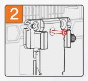
Finally, insert the screw into the middle hole on the upper part of the base and tighten it. The base installation is completed.
