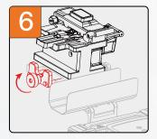
After placing the fiber cleaver on the operating platform, adjust the depth of the screw so that the rubber pad fits the cleaver completely.
