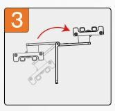
Rotate the support plate to the horizontal position.
