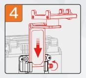
Insert the support plate into the fixing plate and tighten the fixing screws.
