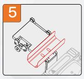
Place the cooling tray in the corresponding position of the support plate, and the installation is completed.
